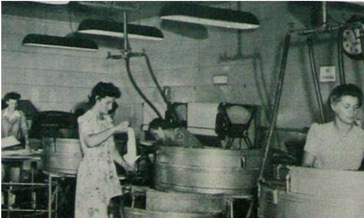
After printing, the pictures are thoroughly washed and dried. Finally, inspectors check and pack the finished prints. All this work from beginning to end is carried in a production line manner.
